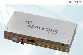
**HiSPiCO** is a transmitter system for S band communication links for small satellites in LEO environment. It is a cost effective, miniaturized, low power solution for CubeSats and achieved TRL 9. The wideband downlink system provides up to 1.6 Mbps at frequencies from 2.1 to 2.5 GHz. Optional matching patch antennas are available.
